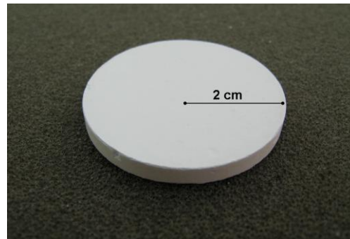
Figure 8. Digital image of a HA/BG_Ca scaffold treated at 750 °C for 3 hours.
