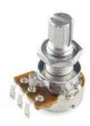
Figure 9: Rotary Potentiometer
