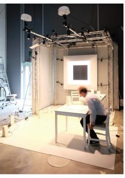
Figure 10. (Top ) Interfaces to the adaptive lighting system, with clear visual, auditive and tactile feedback. The sliders move, the brightness and colour of the screen changes, all adjustments make particular sounds, and when touched, there is tactile feedback. All this to integrate the complex of dynamic changes in the sensibilities of multimodal engagement.
