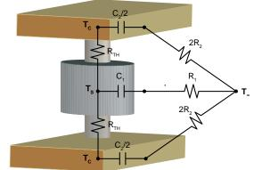
**Figure 2.** The lumped parameter thermal circuit model of the PDCS system during the cooling.
