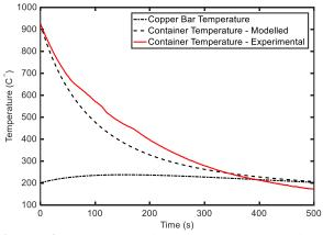
**Figure 4.** PDCS container temperature vs time by simulations for 926°C initial condition.
