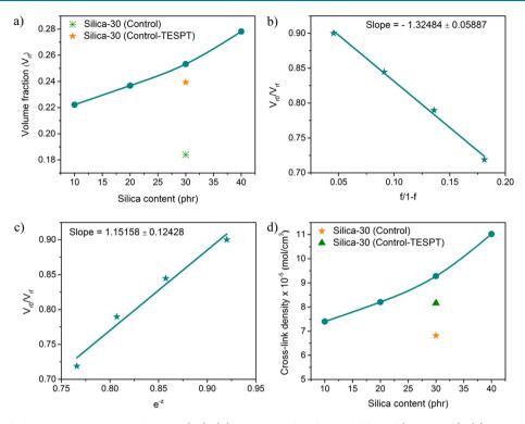
Figure 3. (a) Effect of silica content on volume fraction  $(V_{r_l})$ . (b) Variation of  $V_{r_0}/V_{r_t}$  with f/1 - f (Kraus plot). (c) Variation of  $V_{r_0}/V_{r_t}$  with  $e^{-z}$  (Cunneen and Russel plot). (d) Effect of silica content on cross-link density of silica rubber composites.
