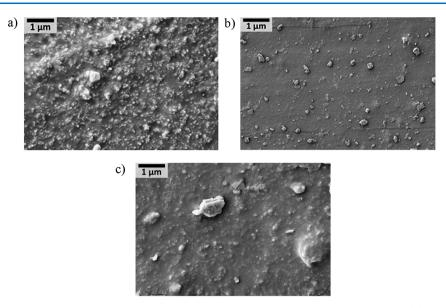
Figure 2. SEM photographs of (a) devulcanized Silica-30, (b) Silica-30 with fresh NR and without silane, and (c) Silica-30 with fresh NR and silane.
