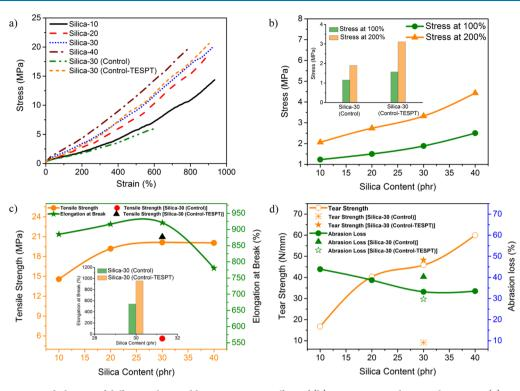
Figure 6. (a) Stress-strain behavior of different silica-rubber composites. Effect of (b) stress at 50 and 100% elongation. (c) Tensile strength and elongation at break. (d) Tear strength and abrasion loss with silica content in the composite.
