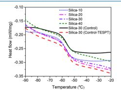
Figure 7. DSC thermograms of different silica rubber composites.
