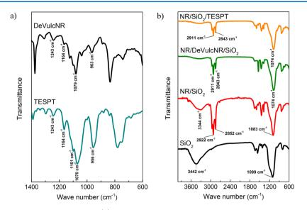
Figure 5. (a) FTIR spectra of TESPT and DeVulcNR; (b) FTIR spectra of SiO<sub>2</sub>, NR/SiO<sub>2</sub>, NR/DeVulcNR/SiO<sub>2</sub>, and NR/SiO<sub>2</sub>/TESPT.
