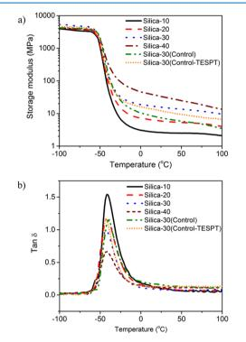
**Figure 8.** (a) Storage modulus and (b) loss tangent ( tan  $\delta$ ) of different rubber–SiO<sub>2</sub> composites as a function of temperature.
