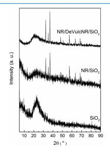
Figure 4. XRD patterns of SiO<sub>2</sub>, NR/SiO<sub>2</sub>, and NR/DeVulcNR/SiO<sub>2</sub>.
