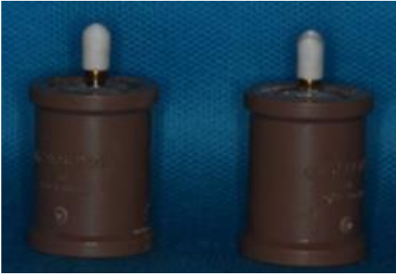
Figure 1. YSZ test specimens of cement-retained implant-supported prostheses.
