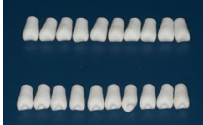
Figure 2. G1 (above) - YSZ without a screw access channel (Control); G2 (below) - YSZ with a screw access channel.
