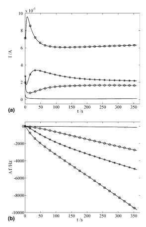
Fig. 3. (a) Chronoamperograms and (b) corresponding  $\Delta f$  vs. t plot in the electropolymerisation of  $3 \times 10^{-3}$  M EDOT in 0.3 M LiClO<sub>4</sub> aqueous solution at (—) +0.75 V, (o) +0.80 V, (\*) +0.85 V and ( $\Box$ ) +0.90 V.
