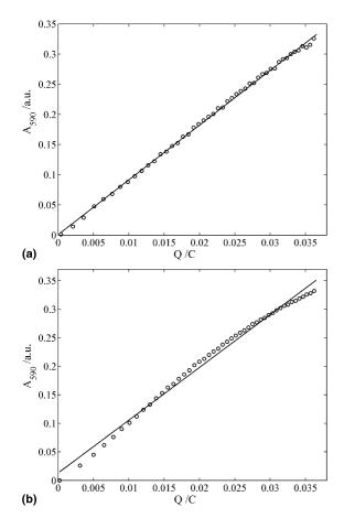
Fig. 7. Absorbance-charge relationships during electropolymerisation of  $3 \times 10^{-3}$  M EDOT in 0.3 M LiClO<sub>4</sub> aqueous solution when the applied potential is (a) +0.95 V during 140 s or (b) +1.05 V during 120 s. Experimental data (o) and data fitted to linear models (—).  $\lambda$  = 590 nm.
