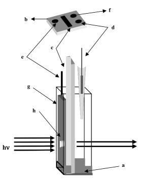
Fig. 1. Schematic diagram of the semi-infinite spectroelectrochemical cell constructed to obtain measurements in normal configuration. (a) Teflon piece with a groove to fix the working electrode, (b) Teflon lid, (c) gold working electrode, (d) Ag/AgCl microreference electrode, (e) platinum auxiliary electrode, (f) hole in the lid to de-aerate, (g) Teflon mask with a 0.5 mm diameter hole (h).
