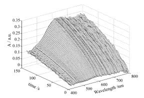
Fig. 5. 3D plot absorbance/time/wavelength in normal spectroelectrochemical arrangement for electropolymerisation of  $3 \times 10^{-3}$  M EDOT in 0.3 M LiClO<sub>4</sub> aqueous solution. E = +0.95 V; t = 140 s.
