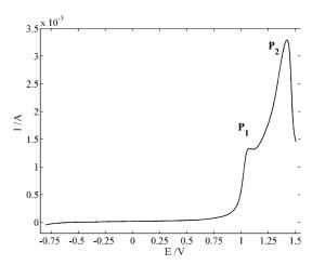
Fig. 2. Linear voltammogram of  $3\times10^{-3}$  M EDOT in 0.3 M LiClO<sub>4</sub> aqueous solution at 0.05 V s<sup>-1</sup> using a gold working electrode.
