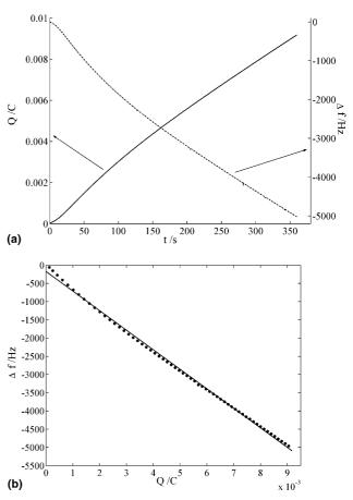
Fig. 4. (a) Q and  $\Delta f$  vs. t plots and (b)  $\Delta f$  it vs. Q relationship during electropolymerisation of  $3 \times 10^{-3}$  M EDOT in 0.3 M LiClO<sub>4</sub> aqueous solution at +0.85 V during 360 s.
