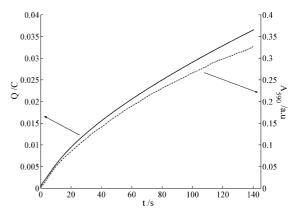
Fig. 6. Absorbance at 590 nm (dotted line) and the corresponding electrical charge collected (continuous line) plotted vs. time. Experimental conditions as in Fig. 5.
