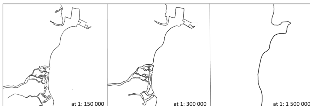
Figure 3.4 Comparison of generalisation of water-channels and shoreline at a different scale (outlines are extracted from hydrographic charts published by the National Hydrographic Office) (for source: refer Appendix, Map-12-14)
