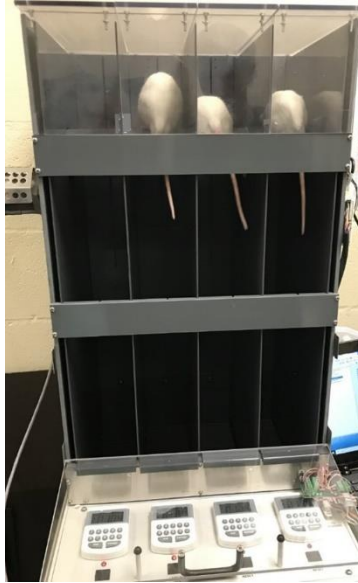
Figure 4.5 Image of an experimental group (includes a high-load impact, low-load impact, and sham rat) walking on the rotating rod of rotarod assay.
