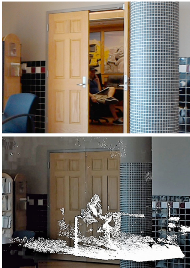
Figure 2.4: An example of a noisy point cloud. Note the boundaryless data and the difficulty localizing the point cloud's position. Image by Christopher Hudson.
