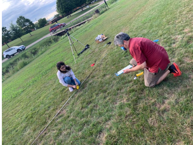
Figure 4.3: Experimenters practicing experimental setup. Tape measures and laser levels were used to set up and validate the experimental area, while the SONIN 10300S ultrasonic depth measurement device was used to measure distances within Experiment 1.
