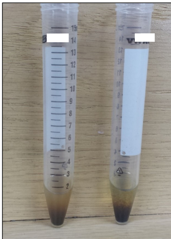
Lemon peel (left) and cloves (right) extracts After one drop of \text{KMnO}_4 solution was added
