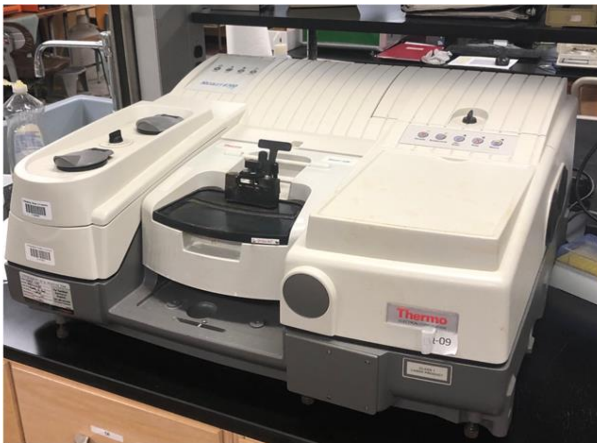
Figure 2.2 Nicolet 6700 FTIR optical spectrometer equipped with a liquid nitrogen-cooled MCT High-D detector, KBr beamsplitter, and Smart ARK accessory
