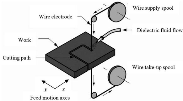
**Figure 1** A typical WEDM process.
