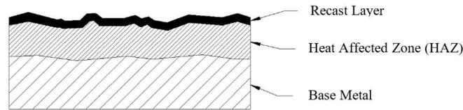
**Figure 5** HAZ below the recast layer.
