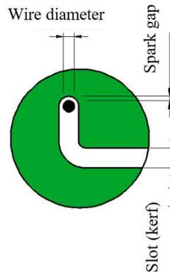
**Figure 4** Details of the spark gap in WEDM.
