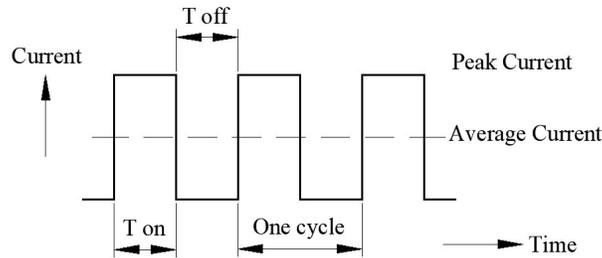
**Figure 3** Relation between WEDM input parameters.
