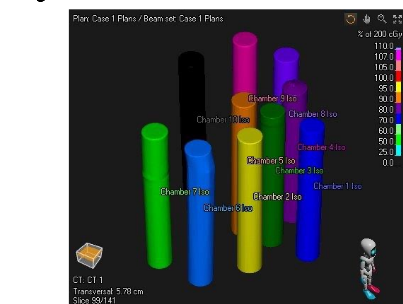
Figure A – 2D CT scan of phantom with each and every phantom insert contoured to highlight the areas of ion chamber insertion Figure B - 3D contours of ion chamber inserts with corresponding isocenters
