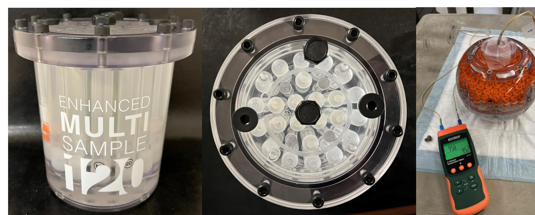
Fig. 3. Cylinder phantom and sphere phantom were constructed as above. Cylinder phantom was used to test that the variables constructed would be able to be scanned properly at a 3T MRI.
