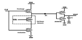
Fig. 1. CMOS Based Domino Buffer
