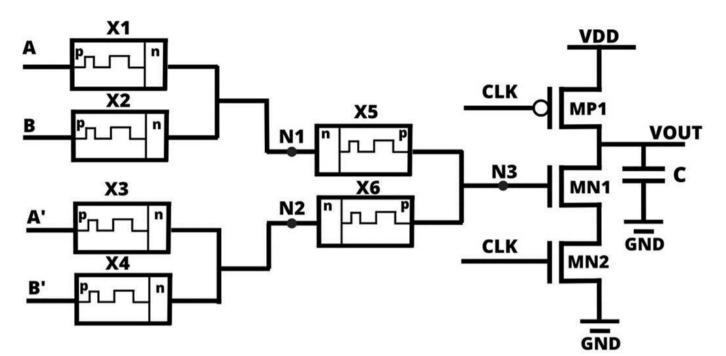
Fig. 7. Proposed Memristor-based Dynamic Exclusive-OR gate
