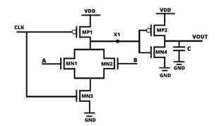
Fig. 2. CMOS based Domino OR gate
