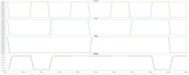
Fig. 8. Timing waveforms for Proposed Memristor-based Dynamic Exclusive-OR gate
