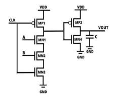
Fig. 3. CMOS based Domino AND gate
