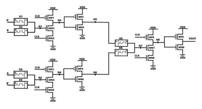
Fig. 6. Existing memristor-based dynamic Exclusive-OR gate
