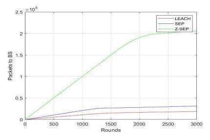
Fig 6: Number of packets to BS in LEACH vs SEP vs Z-SEP
