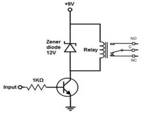
Fig 6: Relay drivers circuit diagram
