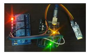
Fig 8(a): Arduino with relay drivers module
