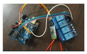
Fig 8(b): Arduino with Bluetooth module
