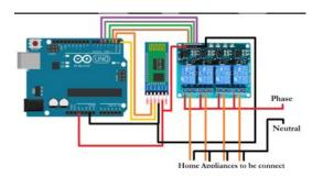
Fig 1 – Circuit diagram of the home automation.
