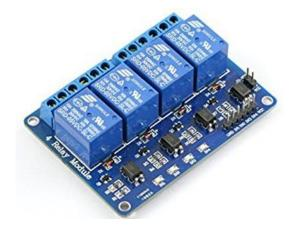
Fig7: Relay drivers module
