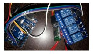
Fig 8(c): Relay drivers module with Bluetooth
