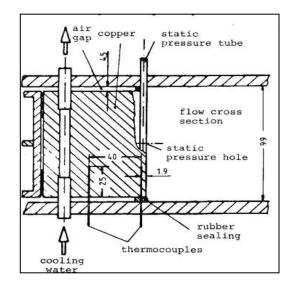
FIG [6] Sectional view; copper
