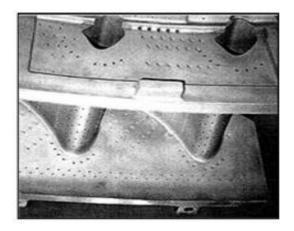
FIG [1] Film cooled turbine vane
