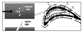
FIG [2] Schematics of typical film cooling configuration, three temperatures potential for film cooled surface
