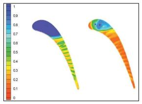
FIG [4] contours of film effectiveness for film cooled tips from pressure side holes for small (left) and large (right) tip gap, both using 0.68% coolant flow measured relative to passage flow
