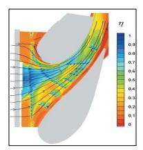
FIG [5] Measured film effectiveness levels for 0.5% slot and 0.5% film cooling flow, flow percentage measured relative to passage flow and predicted streamlines in near wall region
