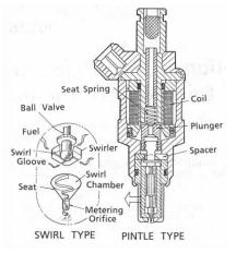
Fig.1 Structure of Injector
