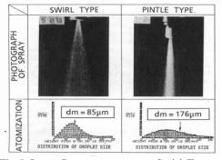
Fig.5 Spray Pattern to compareSwirl Type with Pintle Type **Results**
