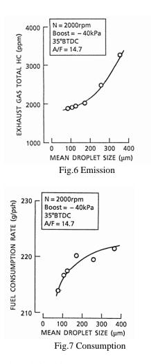
The relationship between the average droplet size of sprayed petrol and fuel consumption is shown in Fig.7. The experimental condition was similar to that of the gas exhaust study above. Fuel consumption rate decreases as droplet size decreases. Depending on the level of fuel consumption in the medium drop size was relatively high.Therefore, when the HC exhaust capacity is limited, the fuel consumption rate is improved.
