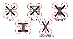
like an H. The arms protrude forth from the body in a direct line. This usually results in a longer body portion to avoid the blades coming into contact with each other. The fact that these frames are so large and the motor position is less flexible for a decent moment of inertia makes them less frequent (due to the long arms).
