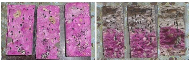
Figure 7 Specimen showing depth of carbonation
