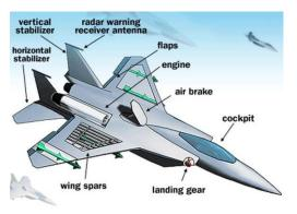
Fig. 3 F16 Components of Aircraft
