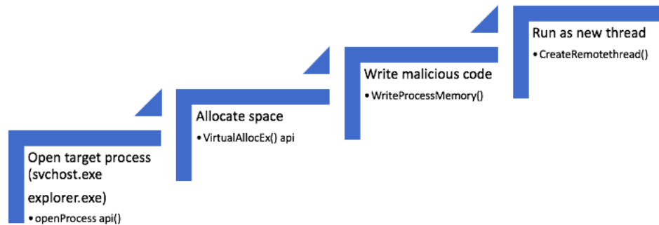
Figure 5: Steps in thread injection
