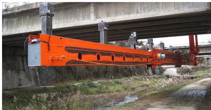
Figure 4. The adjustable boom for image acquisition under bridges [12].
