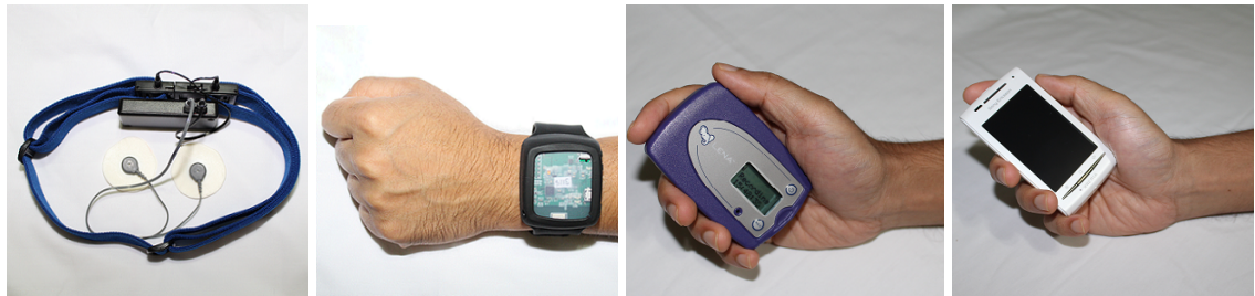
Fig. 3.2: (a) Chest band sensor (captures respiration, ECG, and accelerometer signal). (b) Samrt watch. (c) LENA audio recorder, and (d) Study phone (Sony Ericsson Xperia X10, Android Smart phone).
