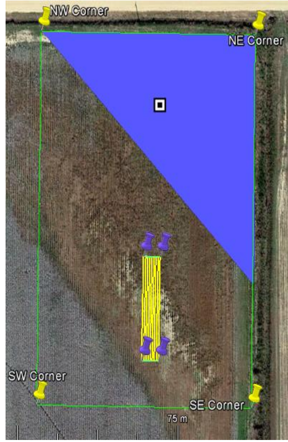
Figure 5: Same as Figure 4 showing the resistivity lines used for the 3-D image within the 100 by 150 meter rectangle. (made using Google Earth)
