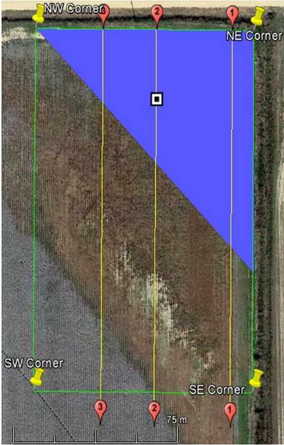
Figure 4: Location of the three resistivity lines. Rectangle is 100 by 150 meters. The white square represents the location of the trench from Cox et al. (2007). Blue triangle marks the conductivity study by Cox et al. (2007). (made using Google Earth)
