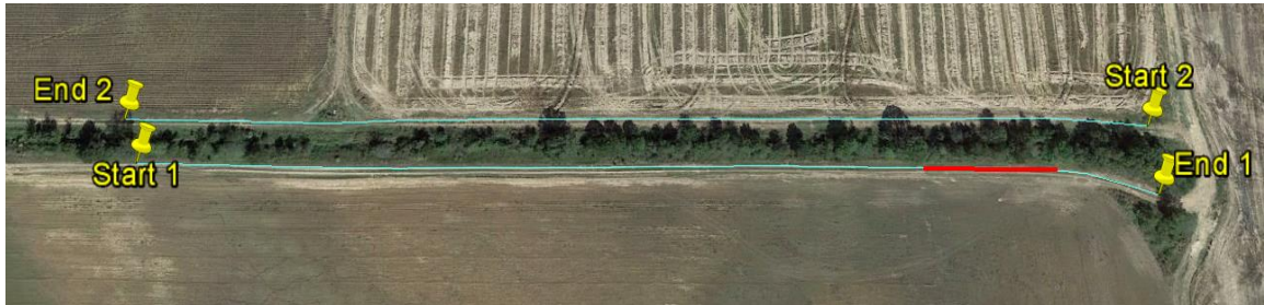
Figure 8: The two 400 meter long GPR lines at Morgan site B. The red line is the data section displayed below (made using Google Earth)
