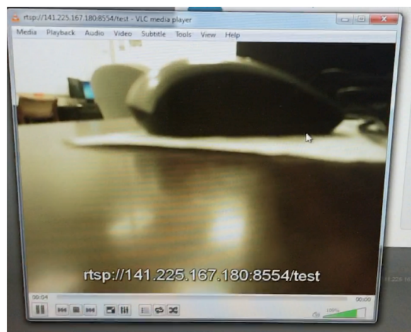
Figure 15: Client PC live streaming of Camera view using rtsp [Real time stream protocol]
