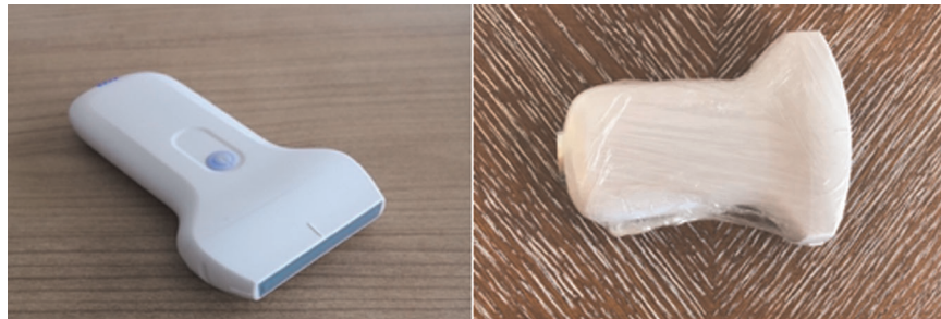
FIGURE 1 Portable wireless linear and convex probes (covered by film) [Color figure can be viewed at wileyonlinelibrary.com ]
