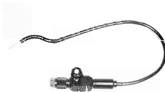
Fig. 3-a. Double-bending Gastrofiberscope (Inaba) 1967. Double-bending mechanism was devised in 1967. This scope was manufactured by the Fuji Photo Optical Co., Ltd., in 1968.
