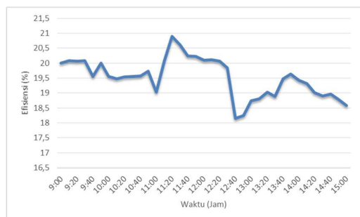
Figure 3.5 Characteristics Efficiency Against Solar Cell Time
