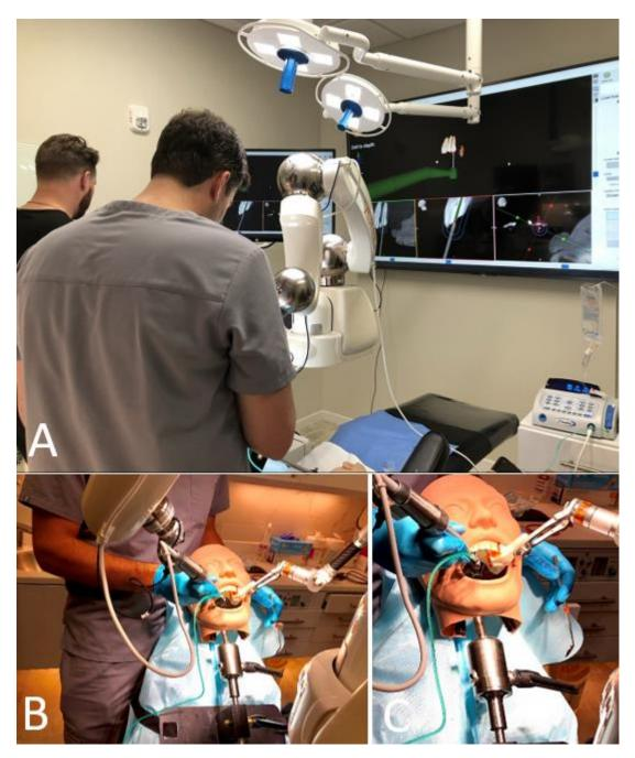
**FIGURE 2.** (A) Overview of robot guided procedure, note clinician is directly viewing operative field with system display being viewed by assistant. (B) Procedure from in front of patient, note the robot kinematic tracking arm in right side of image. (C) Close up of molded Edentulous Patient Splint with kinematic arm attachment in right side of image and drill in use.
