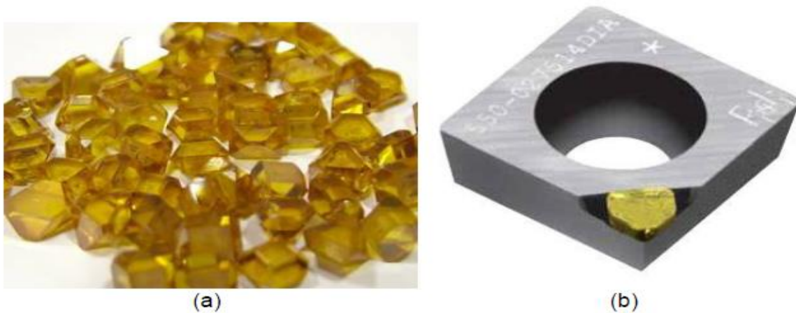
Figure 2.6: Mono-crystalline synthetic diamonds for requiring an ultra-high-quality surface finish (a) manufactured in HTHP processing (b) inserted with mono-crystalline natural diamond cutting edge.
