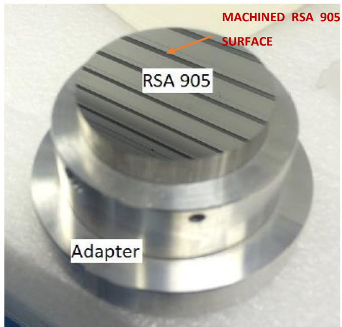
Figure 4.7: Surface of diamond turned RSA 905
