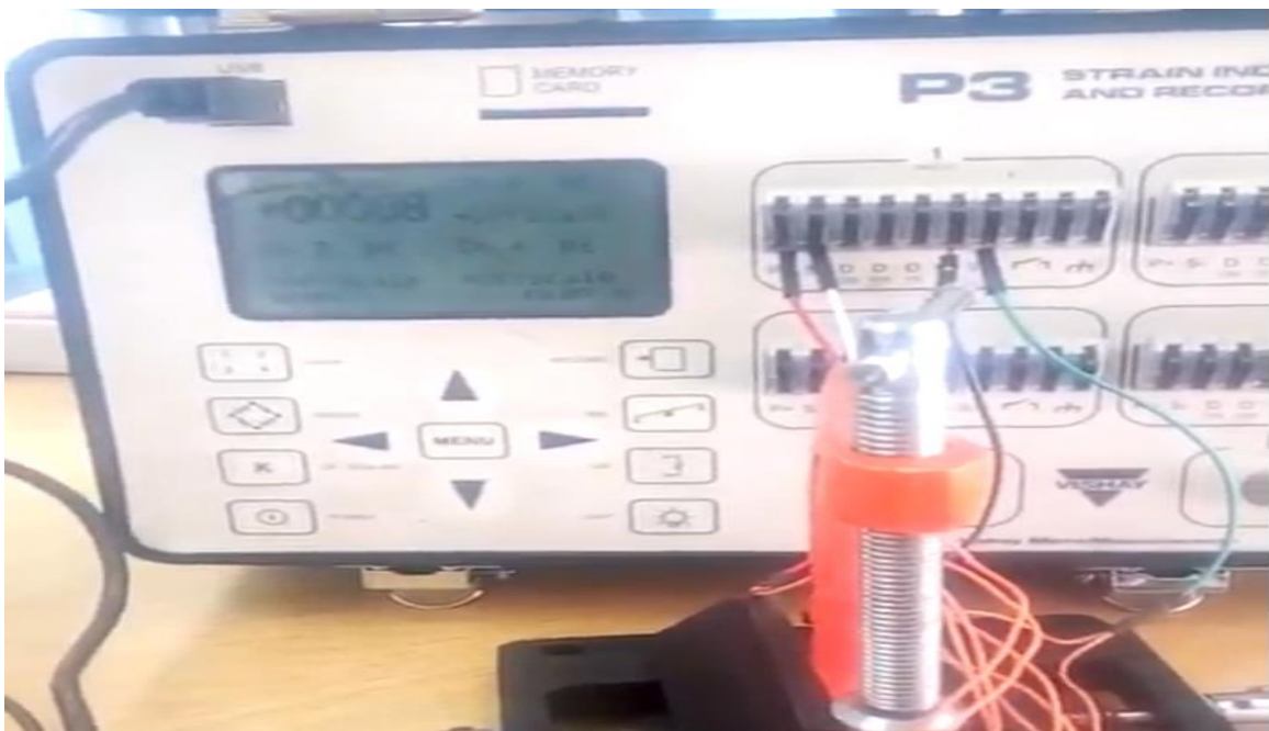
Figure 3.25: Calibration with 125.5g
