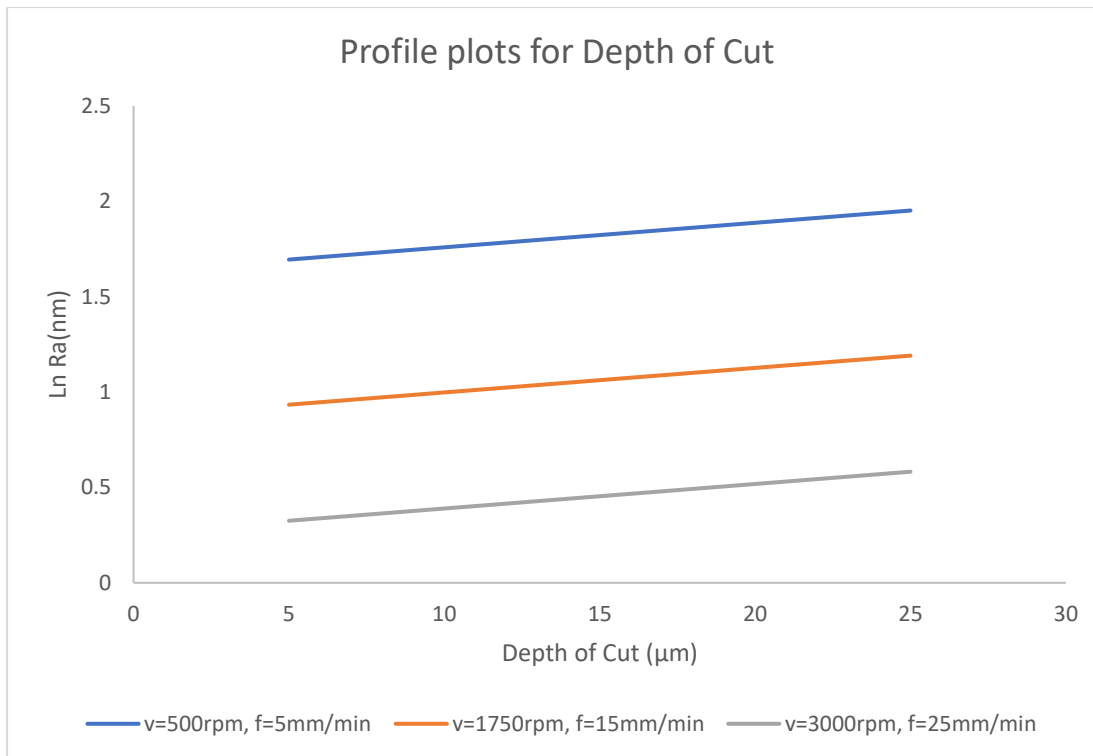
Figure 7.52: Effect of depth of cut on surface roughness at varied feed rates and speed
