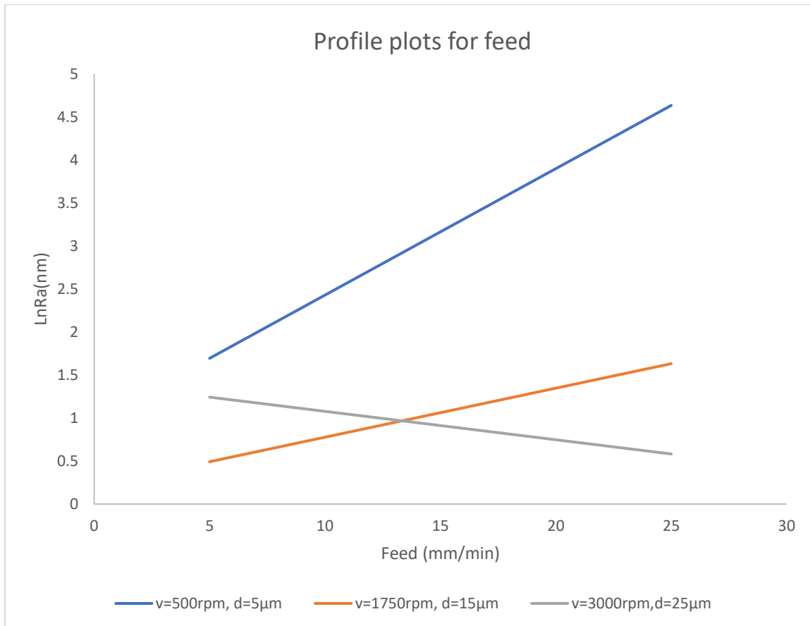
Figure 7.51: Effect of feed on surface roughness at varied speed and depth of cut
