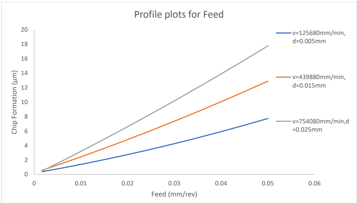
Figure 7.63: Effects of speed on chip thickness at constant feed rates and depth of cut
