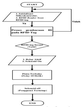
Explanation of locker safety flowchart using RFID.
