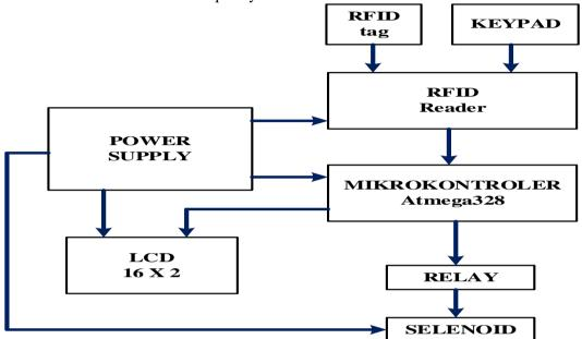
From the block diagram above, you can know a little about the description of this research object and the following is an explanation of the function of each block diagram:
