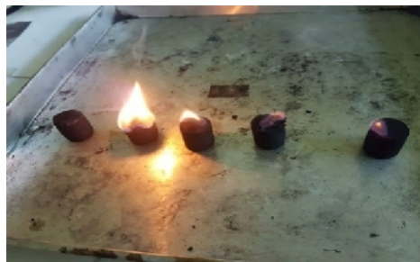
Figure 3. Combustion Rate Test on Biobriquettes
