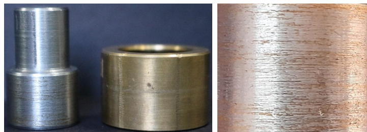
Fig. 7. Pair of assembled parts and shaft surface after disassembling
