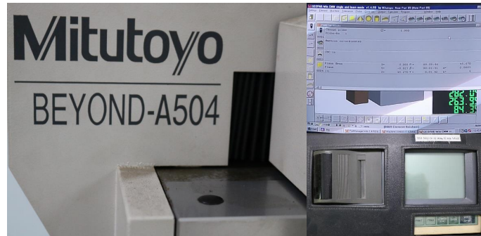
Fig. 2. Coordinate-measuring machine (CMM) and surface profiler
