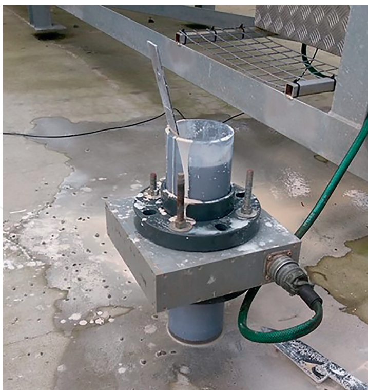
Figure 14. Dummy pipe section for obtaining ERT references of homogenous slurries.
