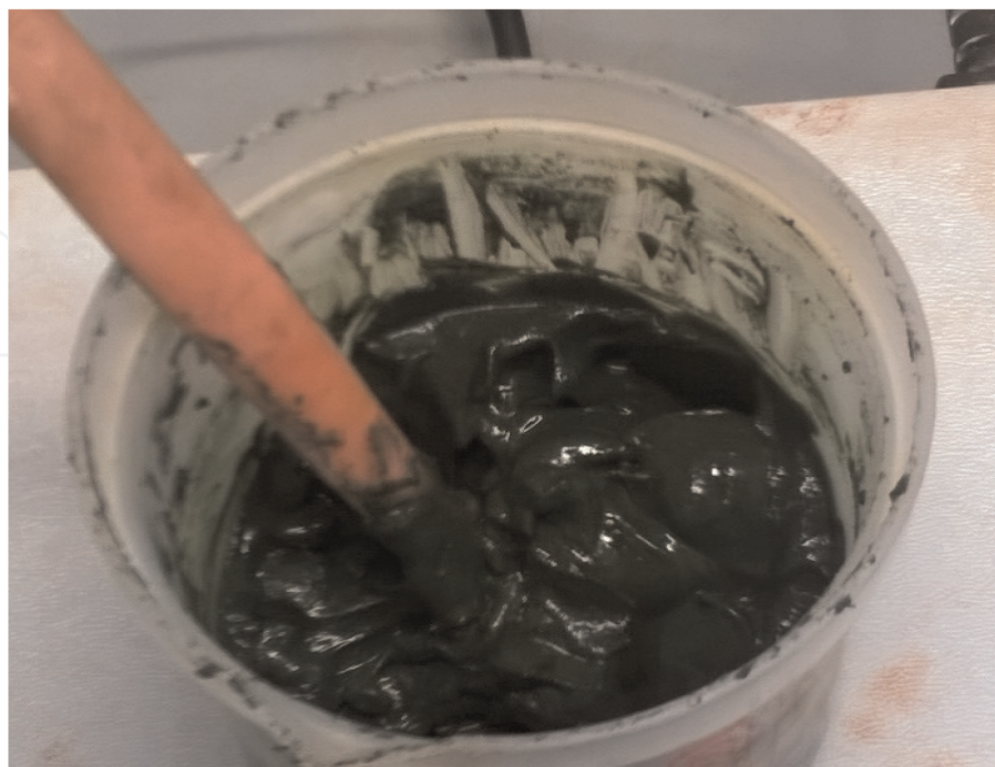
Figure 6. Viscous leach conditions from batch test.
