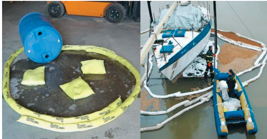
Figure 8. The use of the absorption socks on solid surface (left) and on the water surface (right) [37].
