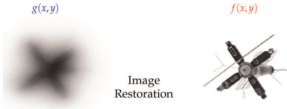
Figure 3. Image deconvolution or restoration inverse problem in satellite imaging.
