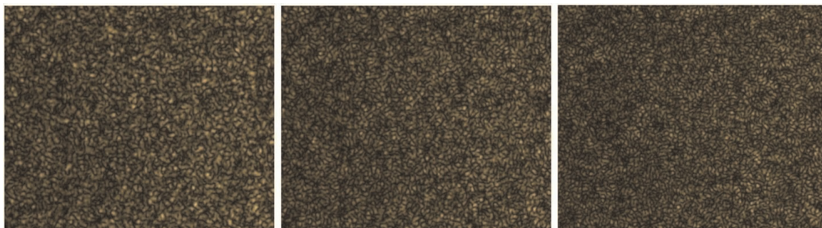
Figure 2. The speckle patterns generated by the scattering of an optical vortex of order +1 (left), order +2 (middle), and order +3 (right) through the ground glass plate.
