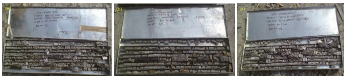
Figure 6. Cores retrieved from the borehole at (a) and (b) powerhouse area; (c) intake drift.
