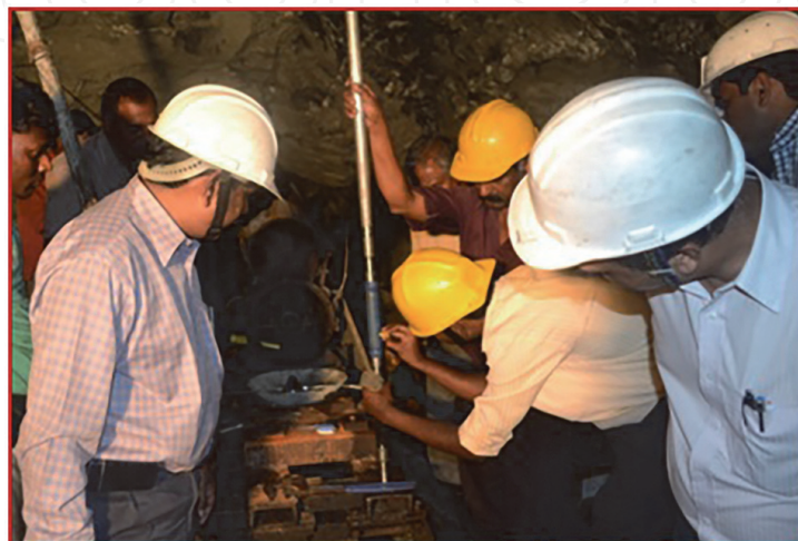
Figure 8. Tracing of fractures from impression packer at powerhouse downstream area.
