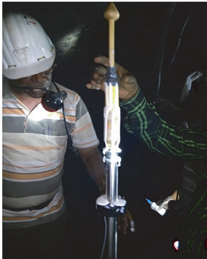
Figure 27. Piston attachment for CISRO HI cell.
