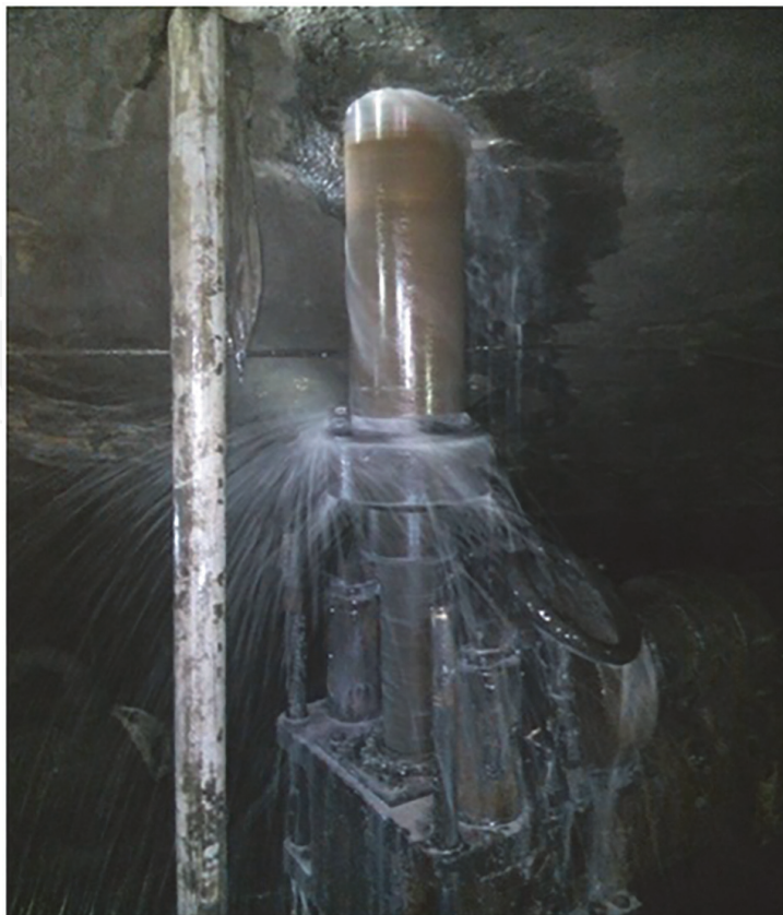
Figure 29. Overcoring test at KTK 8 Incline.
