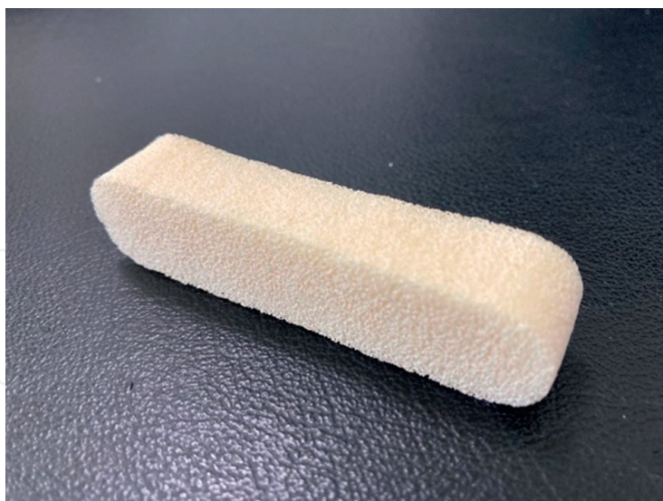
Figure 20. Active tissue-repairing sponges made from chitosan/poly(vinyl alcohol) (Supported by Cenefom and PARSD).
