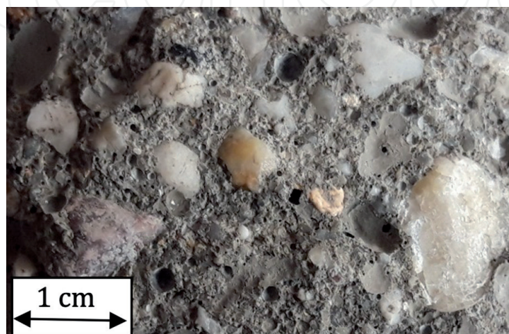
Figure 14. Macroscopic image of the structure of a geopolymer concrete sample.
