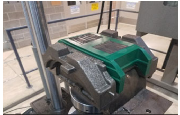
FIGURE 2: POLYMER PAD WITH PROTOTYPE TPU-CNF INSERTS AT THE TWO INTERLOCKS OF THE PAD FOR ENHANCED CONTACT
