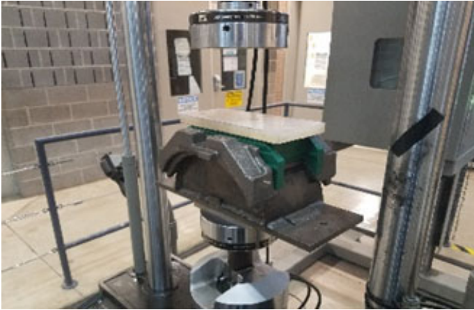
FIGURE 3: MTS 810 MATERIALS TESTER SETUP FOR VALIDATION TESTING OF THE ADAPTER PAD WITH THE PROTOTYPE TPU-CNF INSERTS.
