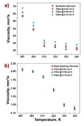
**Figure 3.** Temperature-dependence evaluation for viscosity behavior. (a) SL lubricants; (b) DD lubricants.
