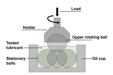
Figure 1. Schematic of four-ball testing setup.
