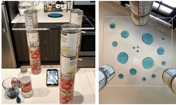
FIG. 3. Left: One of our setups, in the kitchen, with a large droplet of corn syrup dyed blue. Right: Example image showing such several droplets.
