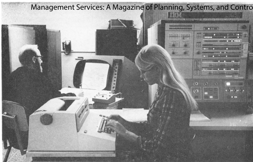
A standard television set has been adapted to serve as a computer graphic display terminal in this experimental system designed by IBM for RAND.
