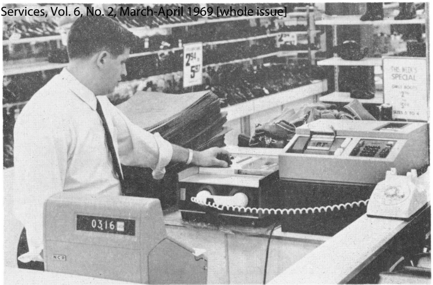
Using Kimball Systems' new SPAN system, a shoe store manager transmits a day's sales statistics to a remote data processing center over telephone lines. The telephone handset is inserted in the cradle of the transmitter.
