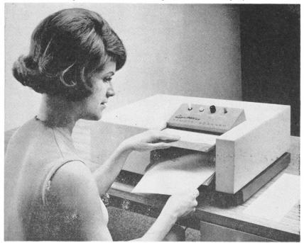
Cognitronics' new desk-top optical scanner occupies less space than an office copying machine. The data scanned are fed by telephone lines to a recognition unit in a Cognitronics service bureau. Separation of the two units and time sharing operation make optical scanning economical for an application that utilizes fewer than a dozen key punch operators, the company claims.
