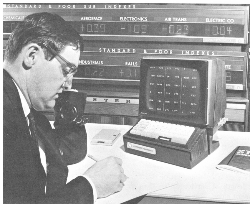
New Ultronic stock quotation machine, in addition to displaying basic stock market quotation data, can monitor any 18 selected securities (as shown above) and alert the broker when one of them hits the price he is waiting for.
